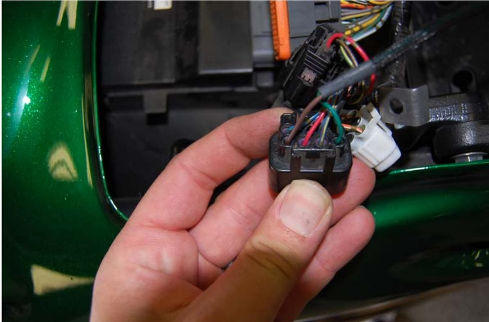
**Once fully installed zip tie the small harness in place to conceal it. Also, it should be mentioned, the Yosh plug should not be used by a Yosh programmer unless you remove the additional wires you just added.**
