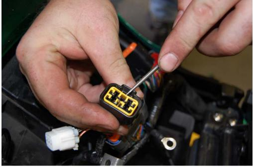
• Insert the brown and blue wires(green in my photo) into their corresponding positions. Brown goes into connector location #8, Blue goes into connector location #5.
