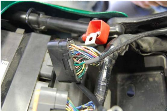
• Unlock your Yosh Connector's yellow lock using a small screw driver or pick.
